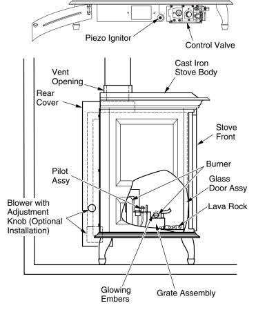
Figure 1 - DESA Direct-Vent Burner System Shown Installed in Approved Cast Iron Stove Body (Oxford™ Model Shown)
